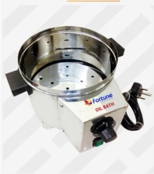
**Application**: Used to heat up Chemical reaction in all labs in Pharma, Chemical, Agricultural and many more.
