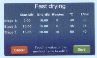
▲ Each method consists of three sectors, allowing control of time, gas temperature, gas flow rate and stage height for each sector.
