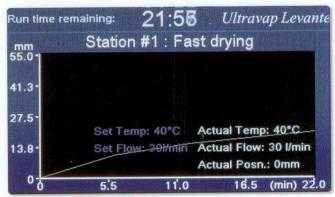
▲ The informative run-time display shows the progress of each evaporation run with real-time information on gas temperature, gas flow rate, stage position and remaining run-time, with an easy to read cursor display.
