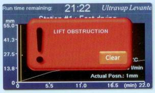
▲ Audible and visual warning of any obstruction is clearly shown and must be cleared by the user or the remote operating system for maximum safety.
